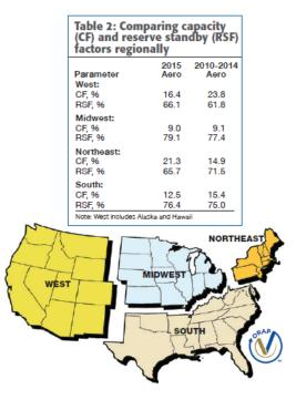
SPS recently prepared for Western Turbine users the latest RAM KPIs from ORAP (Table 1). The company's engineers conducted an exhaustive review of the data and analyzed it for accuracy. The information compiled in the table comes from 627 aero units for 2015 and 1067 units for the 2010-2014 period. The aeroderivative gas turbines in the sample include engines from GE, P&W, and Siemens AGT (formerly Rolls-Royce) and represent units operating worldwide.
